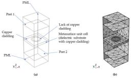
Fig. 3 Example of unit cell of a metasurface and its meshing with triangular basis functions from [3].
